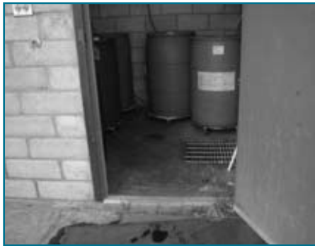
After worksite modification – barrels on wheeled dollies, moved without exertion
