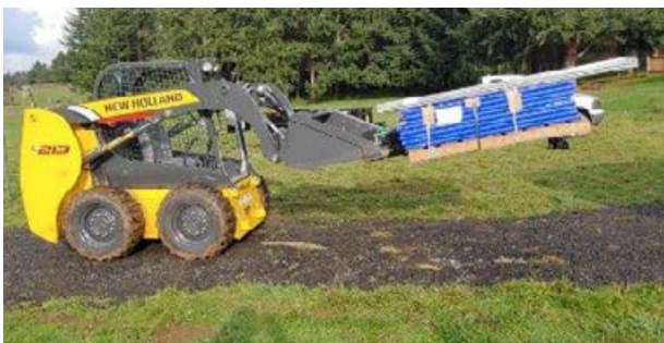
Skid steer loader lifting a pallet with a fork attachment.
