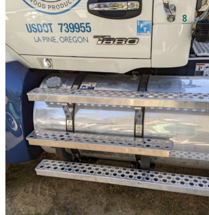
Lowering the steps next to the cab allow easy entry and exit.
