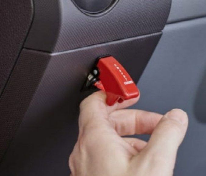
A flip of a switch engages the snow chains.
