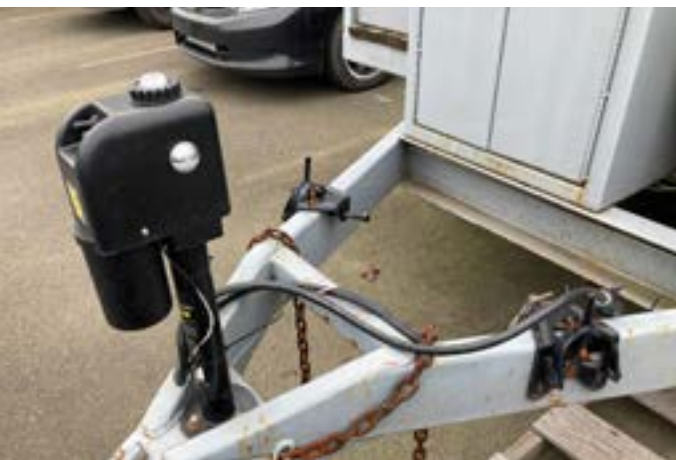
Wallender can now use an electric jack to attach a utility trailer to his work vehicle.
