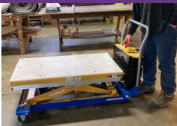
Wallender can use a scissor table and cart to move heavy raw materials.
