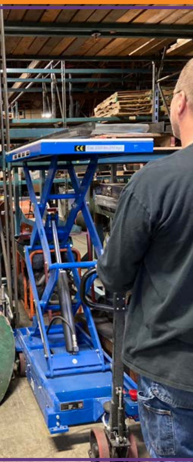
Wallender can use a scissor table and cart to move heavy raw materials.
